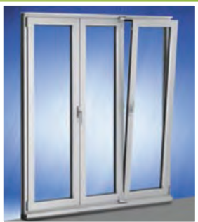
All folding sashes are moved to the side to form a slim package. All 3 to 7 sash units are equipped with an optional Tilt and Turn passage (in-swing or out-swing) door. In the secured tilt position, this sash offers additional possibility of ventilation.
